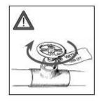
Wasserhaupthahn absperren Close the main water-supply valve
